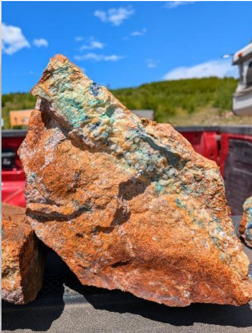
Sample from Ootsa showing quartz vein with malachite, azurite, bornite and native copper.
