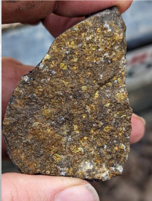
Chalcopyrite fracture-fill from first Ootsa drill hole (3TS-23-34*) which explored under the main showing.
