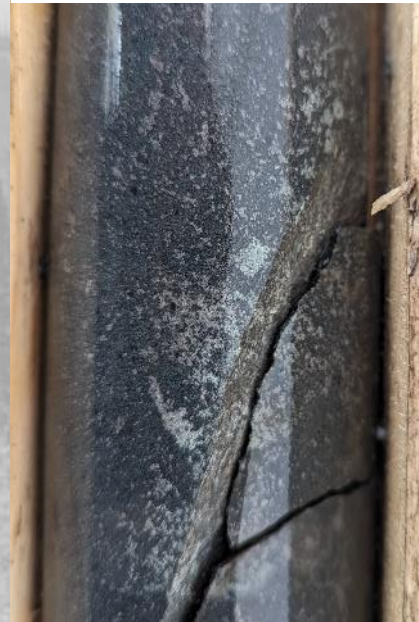
Drill core from inaugural 2023 (3TS-24-34*) drilling with magnetite alteration in microdiorite.
